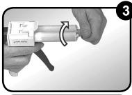
Remove the cartridge cap by rotating the cap 90° in a counter-clockwise direction, then peel away.
