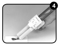
Gently squeeze the dispenser to ensure even flow of both base and catalyst. If this not occur, check for any plugged material and remove with an explorer. Wipe the end of the cartridge clean before installing mix tip.
