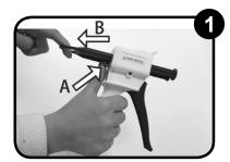
Push the release lever up on the Dispenser (a) and fully retract the plunger (b).
