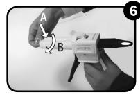
Remove and discard the used mix tip. Replace the cap on the used cartridge and turn the cap clockwise to its locked position.
