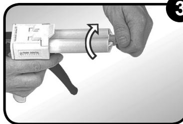
**3** Remove the cartridge cap by rotating the cap 90° in a counter-clockwise direction, then peel away.
