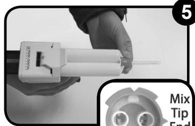
**5** To attach the mix tip: Align the “v-shaped” notch on the mix tip to the “v-shaped” notch located between the cartridge barrels. Push firmly to attach the mix tip to the cartridge.
