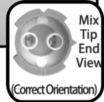
Next, rotate the colored collar of the mix tip 90° in a clockwise direction to its “locked” position. Dispenser is now ready for use.
