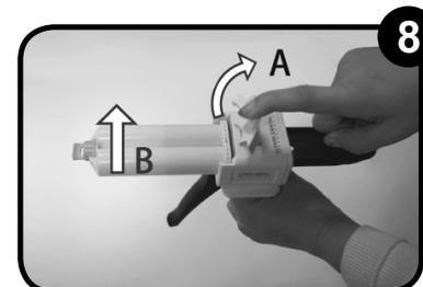
**8** Next, place the cartridge lock in the up position (a), and lift the cartridge out of the dispenser (b).
