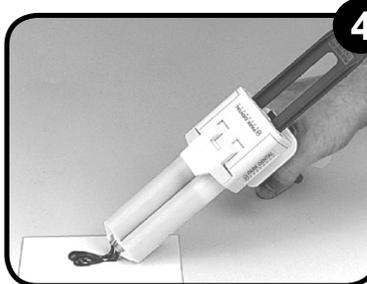
**4** Gently squeeze the dispenser to ensure even flow of both base and catalyst. If this not occur, check for any plugged material and remove with an explorer. Wipe the end of the cartridge clean before installing mix tip.
