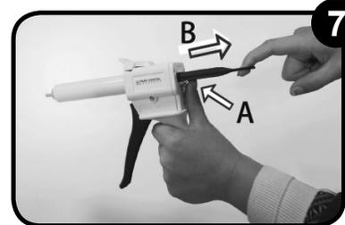
**7** To remove the cartridge: Push the dispenser release lever up (a). Fully retract the plunger (b).
